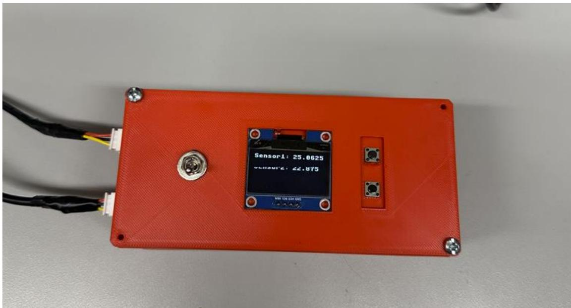
**Figure 5.** Top of third box after implementation. Includes switch, OLED, and buttons. Sensor2 value is distorted from iPhone camera.
